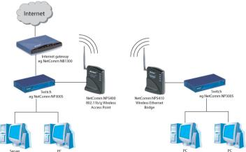
Additionally, the access point enables users on a wireless LAN to access an existing wired network, allowing wireless users to take advantage of the wired networks resources, such as Internet, email, file transfer, and printer sharing.
